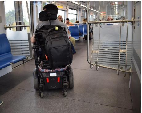
Miami Metro Rail car with transverse seats with handholds on top of seat in left photo and bicycle rack right in right photo and showing stanchions and handrails providing unobstructed space below seats
