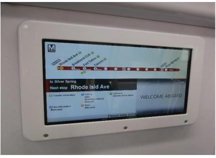
D.C. Metro 7000 series rapid rail cars showing two versions of Real-Time Route Map Tracking displays on D.C. Metro 7000 series rapid rail car.
