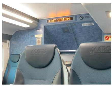
Interior of MARC Bombardier Multi-Level Commuter rail car. Two variable message sign displays showing basic next stop information in different locations in the car.
