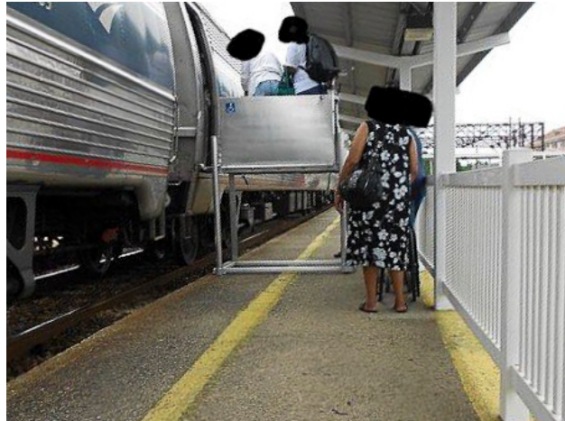
Photo 1: Platform lift in use at Florence station in South Carolina.
